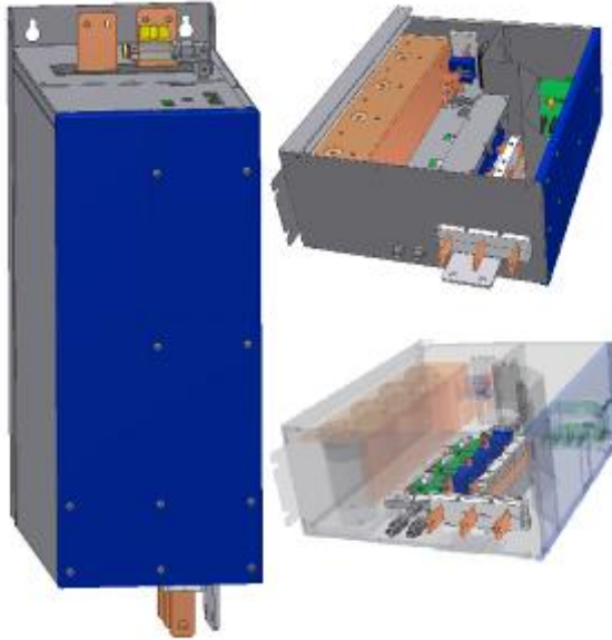
Fig. 4. Sample design solutions the power inverter for the solar plans. The first appearance of the inverter is shown in the basic position. On the other illustrations, there are several views inside the inverter.
