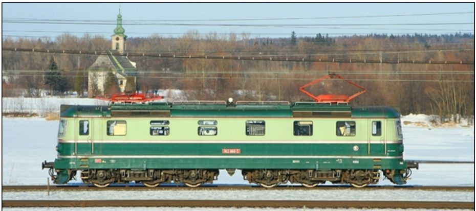
Fig. 2. E669.2 - type locomotive, 3kV voltage, Co 'Co' undercarriage
