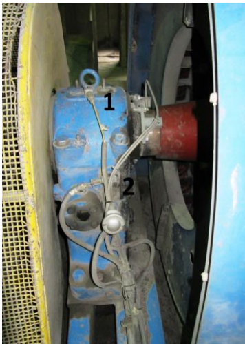
Fig. 3. Measurement accelerometers a) mounted on a bearing stand of an engine, on the drive end, b) sample acceleration meter used in the measurement system – CMSS 2200 [5].
