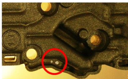
Fig. 6. Lighting two points to measure the height of the object [5]
