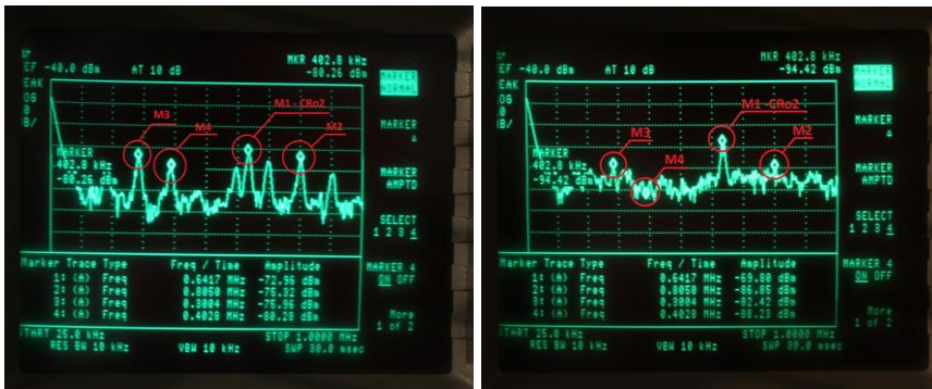
Fig. 5. Measurement of spectrum of magnetization circuit of AMR sensor without and with reduction techniques.
