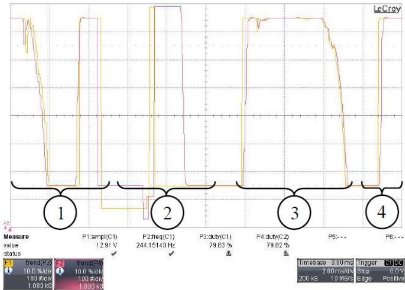
Fig. 5. Measurement of butterfly valves on Audi A6 2.7 TDi
