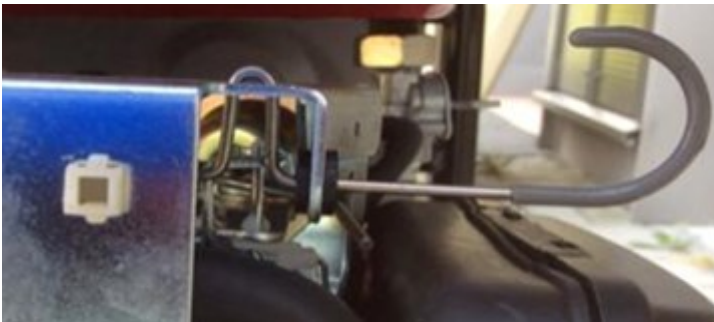
Fig. 2. Combustion engine “choke” in “on” position
