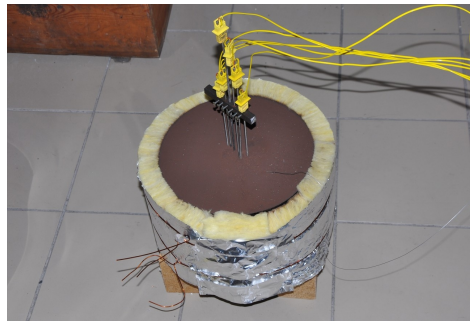
Fig. 2. Steel cylinder with isolation with temperature-sensitive elements.
