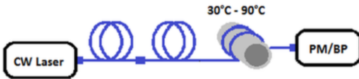
Fig. 1. The beam profile and the output power measurement diagram.
