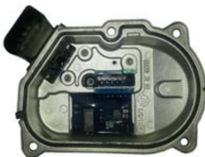
Fig. 4. Photo of actuator control electronics of butterfly valves
