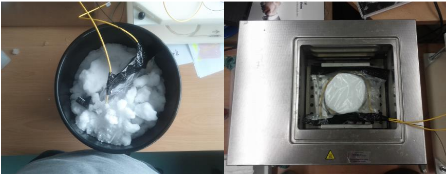
Fig. 3. Testing erbium doped fiber IsoGain I-6 at 1°C temperature and 50°C
