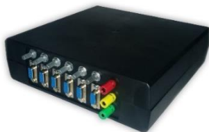
Fig. 3. Multichannel photoplethysmography device with three connectors for ECG electrodes. ECG is in this device use as time synchronization of all of pulse wave during one cardiac cycle.
