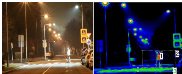
Fig. 4. Photo of zebra crossing and luminance analysis
