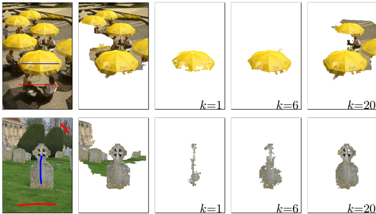
Fig. 5. On the influence of the k value on the segmentation result. The input images with the seeds (the first column), the results of segmentation based on the geodesic distance (the second column), and the results of segmentation based on the k -max distance for various values of k (the columns 3-5).
