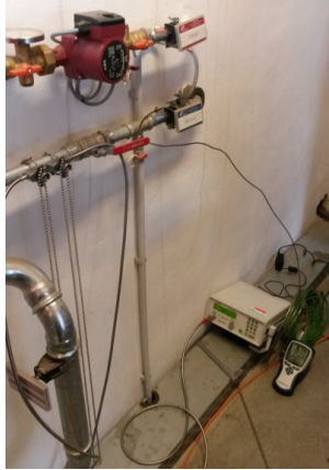
Figure 1. Measurement gauges connected to measure consumption of heat flowing into the biogas processing plant
