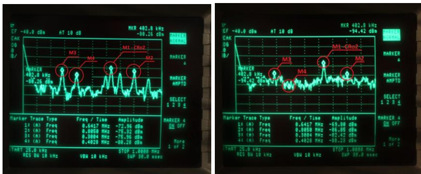
Fig. 3. Measurement of spectrum of magnetization circuit without and with reduction techniques.
