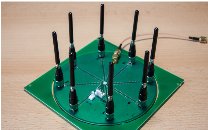
Fig. 2. Pseudo-Doppler antenna array
