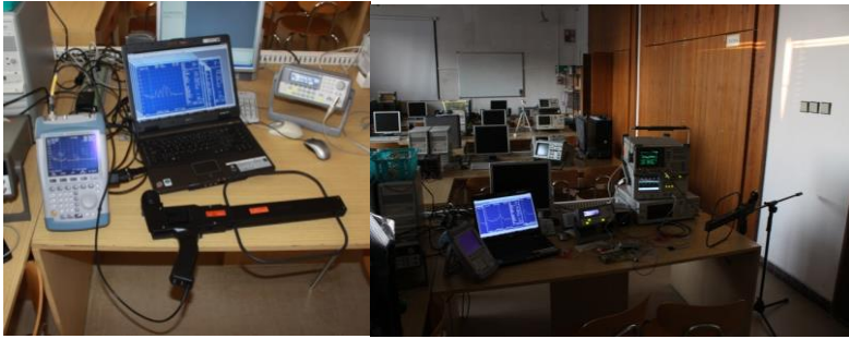
Fig. 2. Measurement equipment and workplace for measurement of electromagnetic radiation
