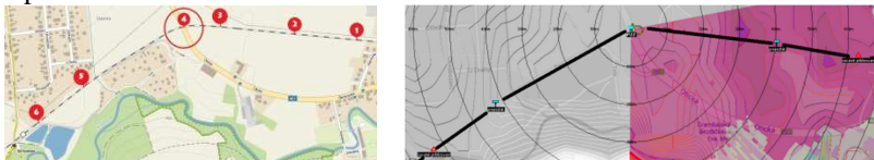
Fig. 4. Map of the testing LCSD Otice u Opavy and one part of the radio propagation model.
