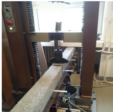
Fig. 2. Measuring system composed from FP 10 device, cementitious sample and optical fiber.
