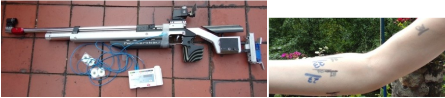
Fig. 2. Left: SOMNOScreen device and air rifle prepared for measurement. Right: shooter's arm with marks for attaching electrodes
