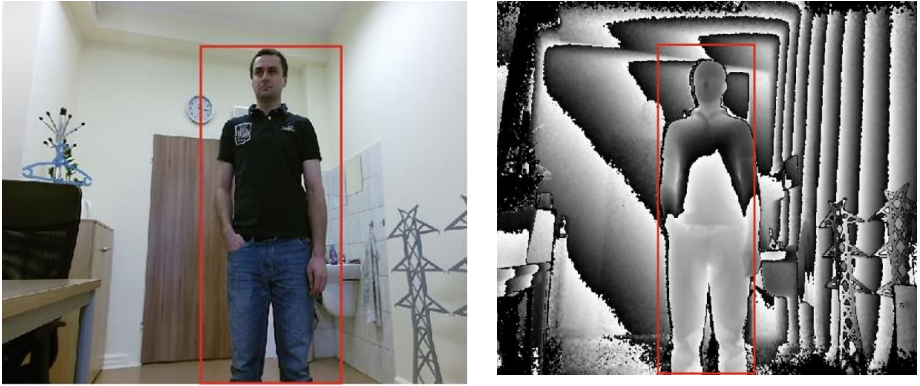
Fig. 2. The result of the program: silhouette detected in the RGB picture and depth on the map
