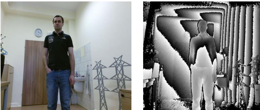
Fig. 1. RGB image to the left and depth map to the right
