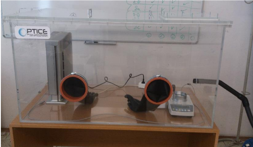
Fig. 4: Picture of created vacuum box
