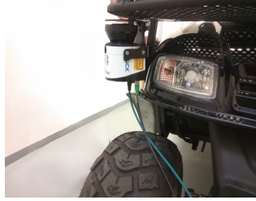
Fig. 2: Placement of LIDAR on the vehicle
