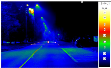
Fig. 4. A luminance analysis of the road with LED luminaires (direction 1) [6]
