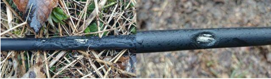
Fig. 1. Insulation, damaged by PD activity
