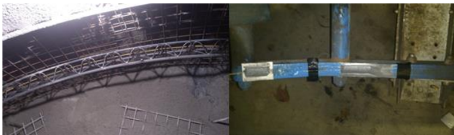
Fig. 7: Implementation of optical fiber for deformation monitoring in the tunnel (left) and application of FBG sensor on mechanical construction of the garbage truck for dynamically weighing of municipal waste (right).
