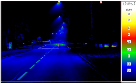
Fig. 5. A luminance analysis of the road with LED luminaires (direction 2) [6]
