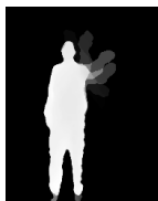
Fig. 2. The demonstration of the 30th frame of the first action stream from MSR Action3D Dataset where the Gaussian blurring is applied across the time. The ghosts of short history and future are seen here.
