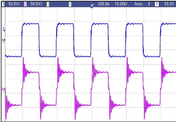
Fig. 6. Waveforms of primary AC link transformer winding voltage (blue curve, V) – and secondary AC link transformer winding voltage (violet curve, V), obtained from AC link DC-DC converter realized model, taken from [3]
