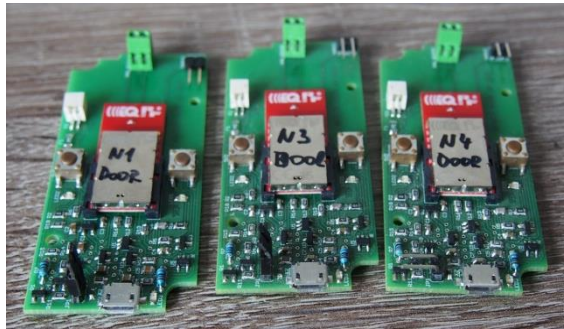
Fig. 4. The wireless devices for detection of entry
