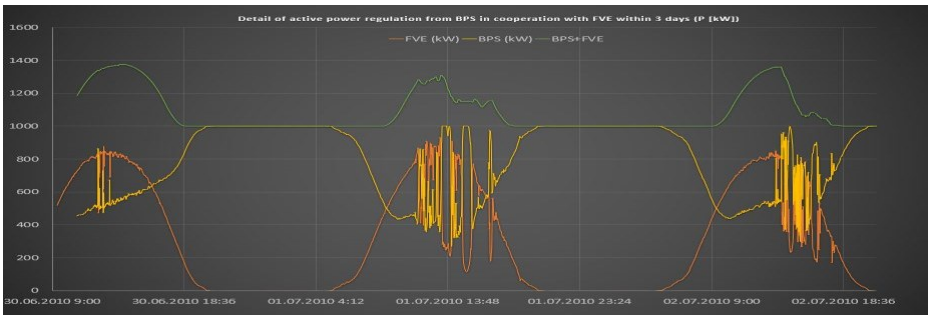
Fig. 3. Theoretical course of total active power from both sources to one DS point
