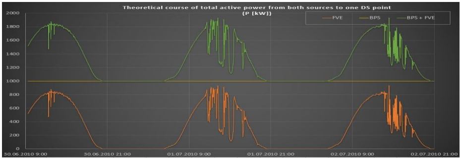
Fig. 2. Theoretical course of total active power from both sources to one DS point
