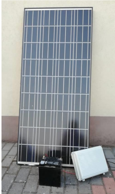
Fig. 3. Air measurement unit with cryptocurrency mining machine (uP PC) [9]
