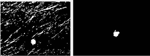
Fig. 5. Input (left) and output (right) of the erosion method.
