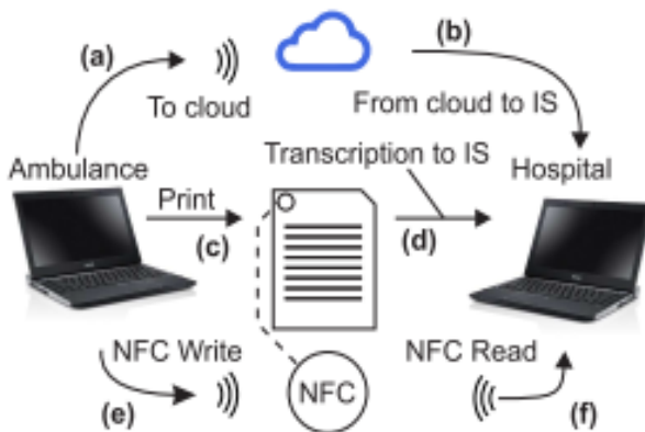
Fig. 2. Scheme of information transfer between the EMS and the hospital the patient is transported to.
