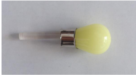
Fig. 2: An incandescent lamp made from PDMS.
