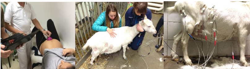
Fig. 2. The verification of the fPCG measurement system on human and animal subject.
