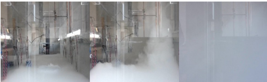
Fig. 2. The creation process of fog by sublimation of the dry ice (carbon dioxide \text{CO}_2 gas).
