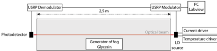
Fig. 1. Measurement of fog influence on FSO link.
