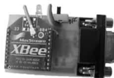
Fig. 5. ChipOx node (bottom side) with XBee
