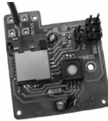
Fig. 1. Tire Sensor board (sensor + MCU-transmitter, BDM, serial line), battery from the bottom, antenna on the top
