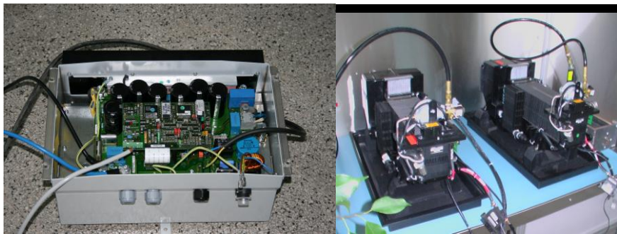
Fig. 5. On the left: Inverter Sunnyboy, On the right: Two connected Nexa modules in digester.
