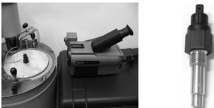
Figure 2. a) The measuring by the infrared camera. b) Picture of bimetallic thermometer.
