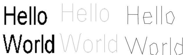
**Fig. 3.** Input binary image along with its thinned form and refined vector result containing  $n = 18$  polylines.
