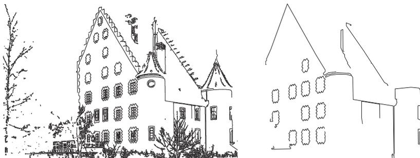
**Fig. 5.** The first picture shows line drawing containing  $n = 12,617$  polylines made of  $m = 38,433$  line segments. In second picture is the result of vector removal component (with *upperbound* = 20) combined with Douglas-Peucker simplification. The output contains  $n = 19$  polylines with  $m = 473$  line segments.
