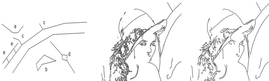
**Fig. 4.** The first picture gives example of the most typical small artifacts – **a.** unconnected polylines **b.** insignificant cycles **c.** 1-connected polylines **d.** spurious loops **e.** insignificant junction connections. The second picture shows an input vectorized image. On the third picture there is output of the artifact removal component (configured to ignore short artifacts) and Douglas-Peucker polyline simplification algorithm.
