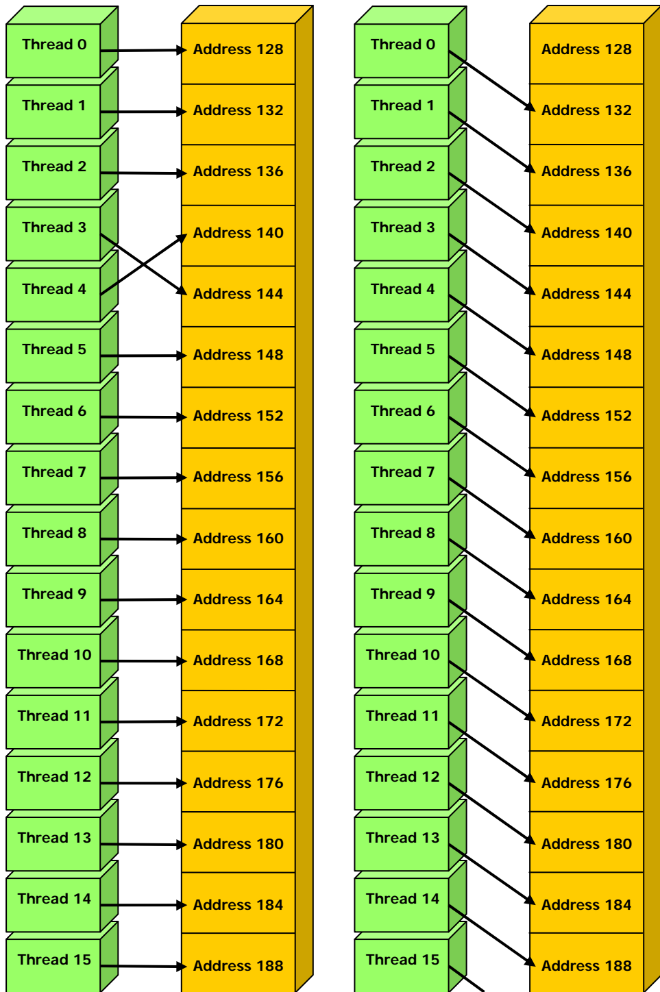
Left: non-sequential float memory access, resulting in 16 memory transactions. Right: access with a misaligned starting address, resulting in 16 memory transactions.
